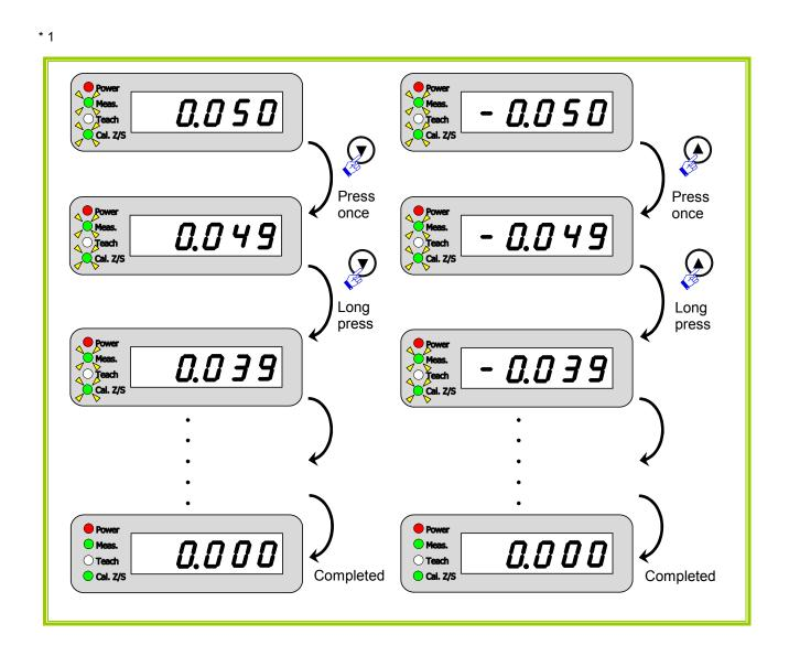
• Setting the runout center to 0 V
