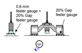
5 Set the sensor gap to 20% and press the "Set" button on the converter. <sup>\*1</sup>
