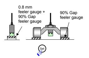
21 Set the sensor gap to 90% and press the "Set" button on the converter. <sup>\*14</sup>
