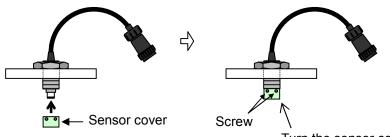
Turn the sensor cover to attach it. After attaching the sensor cover, tighten the screws.
