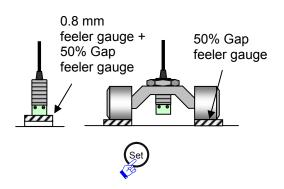
**13** Set the sensor gap to 50% and press the "Set" button on the converter. <sup>\*10</sup>
