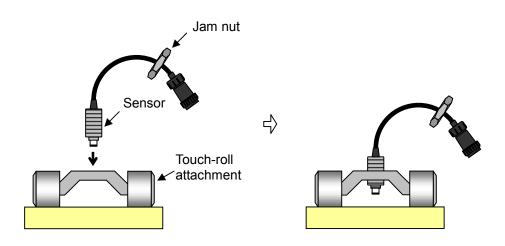
3 Insert a 0.8 mm feeler gauge between the sensor tip and the target and adjust the position of the sensor.
