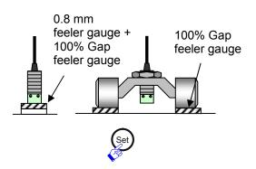
23 Set the sensor gap to 100% and press the "Set" button on the converter. <sup>\*15</sup>
