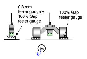
7 Set the sensor gap to 100% and press the "Set" button on the converter. <sup>\*3</sup>
