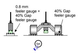
Set the sensor gap to 40% and press the "Set" button on the converter. <sup>\*2</sup>
