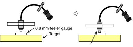
Turn the sensor body and let the sensor tip touch the 0.8 mm feeler gauge. Be careful not to damage the sensor tip. **4** Fix the sensor in place by tightening the jam nut.
