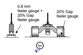
7 Set the sensor gap to 20% and press the "Set" button on the converter. <sup>\*7</sup>
