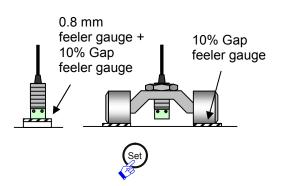
5 Set the sensor gap to 10% and press the "Set" button on the converter. <sup>\*6</sup>
