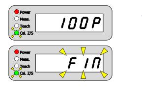
8 The seven-segment LED display will show "100P" (1.5 seconds), and then flash indicate "FIN".
