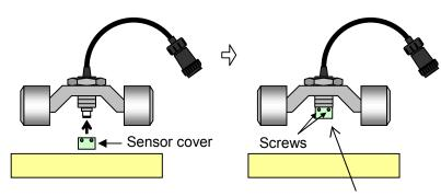
Turn the sensor cover to attach it. After attaching the sensor cover, tighten the screws.
