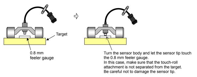
**4** Fix the sensor in place by tightening the jam nut.
