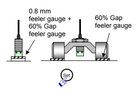
9 Set the sensor gap to 60% and press the "Set" button on the converter. \*<sup>3</sup>
