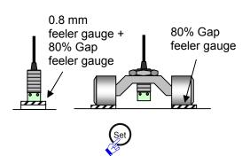
**11** Set the sensor gap to 80% and press the "Set" button on the converter. <sup>\*4</sup>
