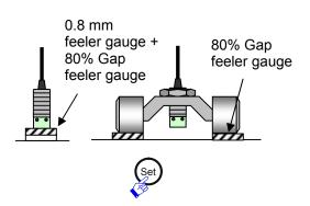
**19** Set the sensor gap to 80% and press the "Set" button on the converter. <sup>\*13</sup>
