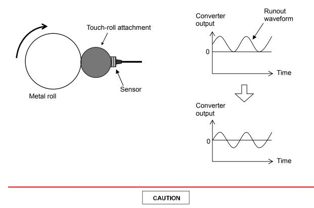
When performing a plating process on the metal roll (target), unevenness in the plating thickness may appear in the converter output (electrical runout).
