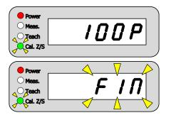
6 The seven-segment LED display will show "100P" (1.5 seconds), and then flash indicate "FIN".
