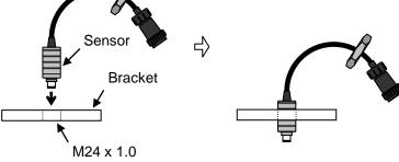
3 Insert a 0.8 mm feeler gauge between the sensor tip and the target and adjust the position of the sensor.
