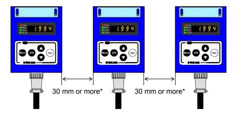
\* If the ambient temperature exceeds 40°C, it is recommended that you maintain a space of at least 50 mm (approximate) around the converter.
