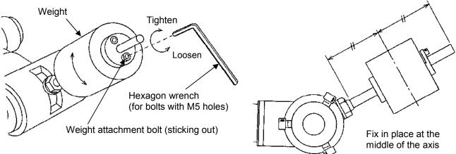
Loosen the weight attachment bolt to turn the weight
