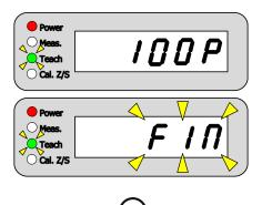
14 The seven-segment LED display will show"100P" (1.5 seconds), and then flash indicate"FIN".
