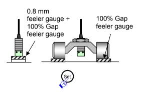
**13** Set the sensor gap to 100% and press the "Set" button on the converter. <sup>\*5</sup>
