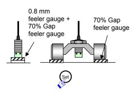
**17** Set the sensor gap to 70% and press the "Set" button on the converter. <sup>\*12</sup>
