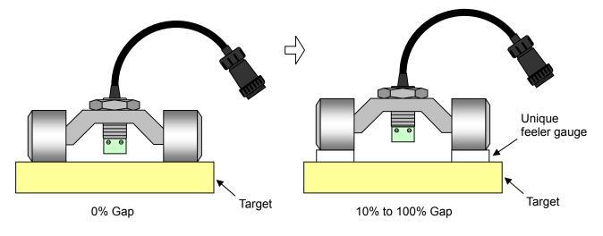
When the touch-roll attachment is used, you can use not only a non-metallic feeler gauge, but also a feeler gauge made of magnetic or conductive material such as metal.
