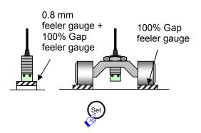
5 Set the sensor gap to 100% and press the "Set" button on the converter. <sup>\*1</sup>
