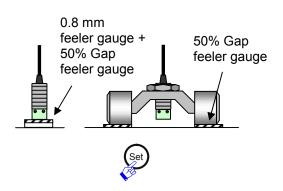
${\bf 5}$  Set the sensor gap to 50% and press the "Set" button on the converter.  $^{*2}$
