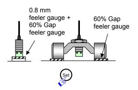
**15** Set the sensor gap to 60% and press the "Set" button on the converter. <sup>\*11</sup>
