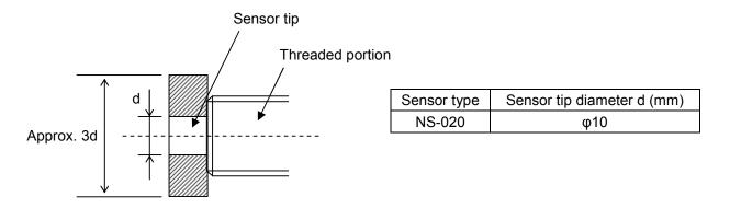
You need to be careful if you are using a jig other than the special attachment since there are cases where performance is decreased if conductors such as metals are present in the
