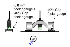
**11** Set the sensor gap to 40% and press the "Set" button on the converter. \*9
