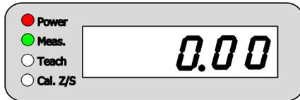
**27** When adjustment is completed, the mode will change to the measurement mode.
